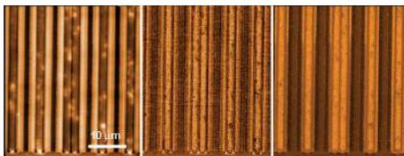
SMM images of simultaneous topography, capacitance, and dC/dV images of SiGe transistor device.
