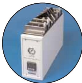
Micro-Chamber/Thermal Extractor ( \mu -CTE) for measuring emissions from materials & consumer products
