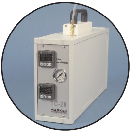
TC-20 multi-tube conditioning/dry purge unit for up to 20 tubes
