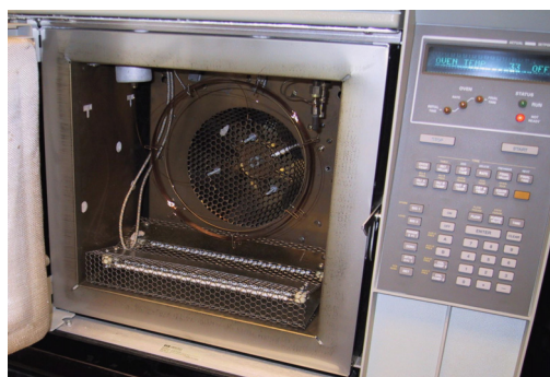
Figure 1. GC Racer Heater installed on an Agilent 5890 GC
