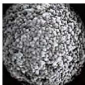
ZORBAX Rx-SIL uniform sub particles
