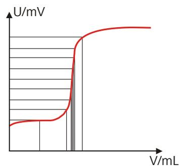
Figure 14 Reagent dosing for DET
