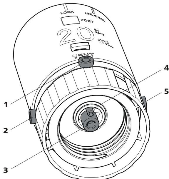
Figure 17 Dosing unit – port assignment
