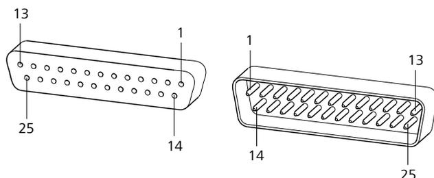
Figure 29 Pin assignment of remote socket and plug
