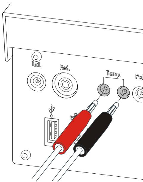
Figure 10 Connecting a temperature sensor or an electrode with integrated temperature sensor
