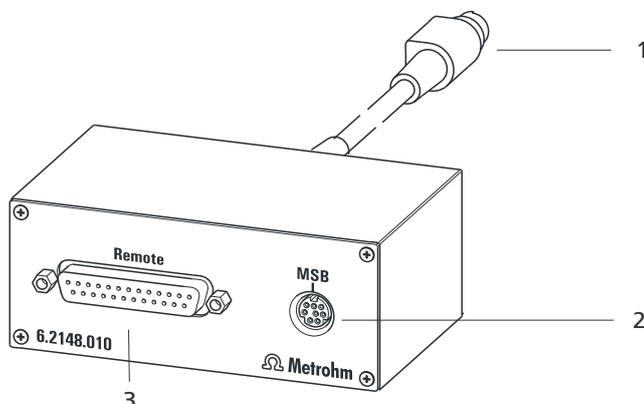
Figure 28 Connectors of the Remote Box
