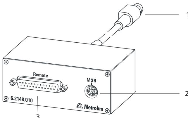
Figure 28 Connectors of the Remote Box
