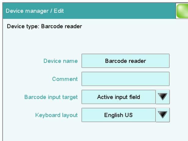
A barcode reader can be connected to read in sample data or other texts. A connected barcode reader will be recognized automatically and entered in the list of devices with default settings.
