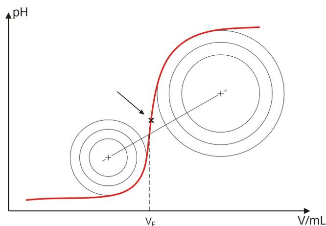
Figure 22 Tubbs method for determining the equivalence point
