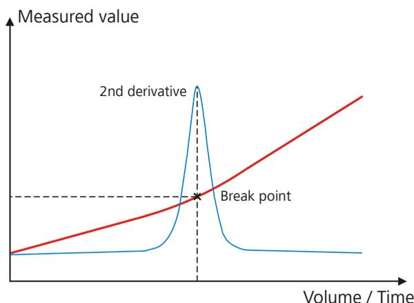
Figure 26 Evaluation of a break point
