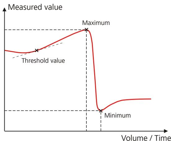
Figure 25 Evaluation of minimum and maximum
