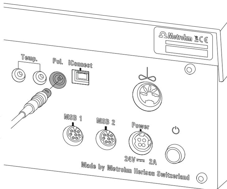
Figure 9 Connecting a polarizable electrode
