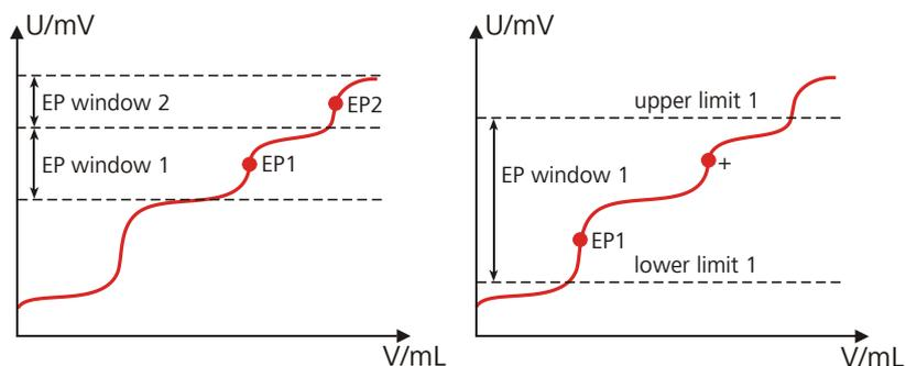
Figure 23 Equivalence point recognition and equivalence point numbering within windows
