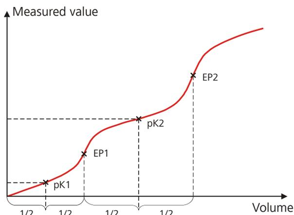
Figure 24 Evaluation of pK value / half neutralization potential
