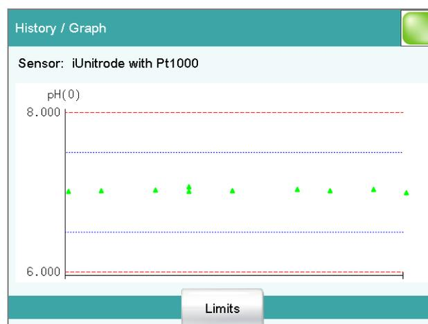
In this diagram, either slope or pH(0) is plotted against the date of the calibration. You can define warning limits (blue dashed lines) and intervention limits (red dashed lines). These limits will not, however, be monitored.
