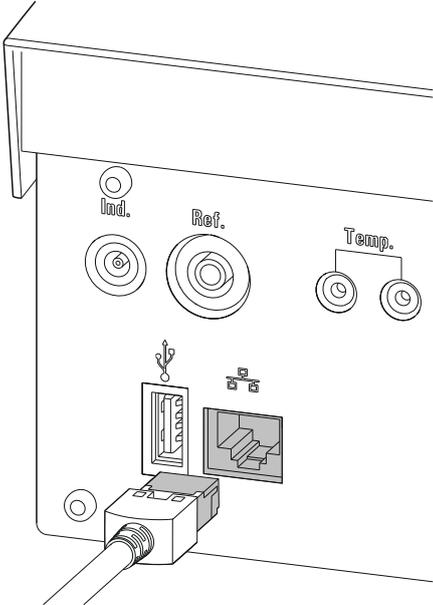
Figure 13 Connecting the Ti-Touch to a network
