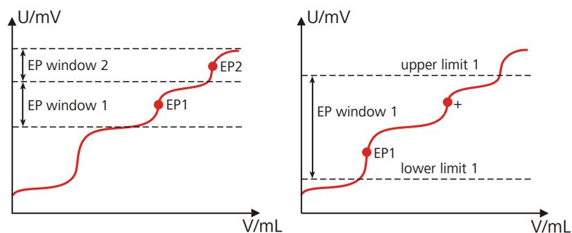
Figure 21 Equivalence point recognition and equivalence point numbering within windows
