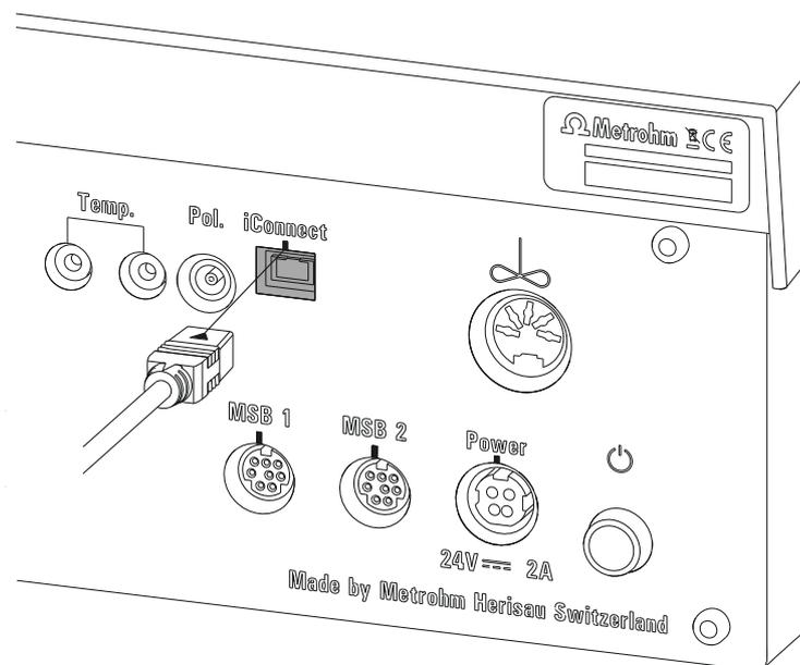
Figure 11 Connecting the iConnect
