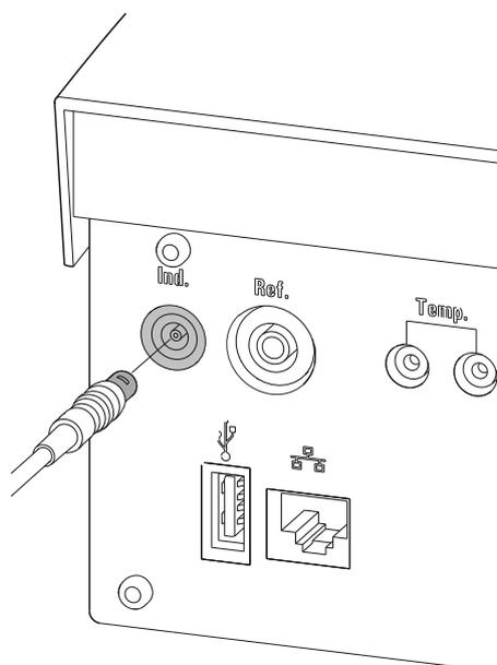
Figure 7 Connecting a pH, metal or ion-selective electrode
