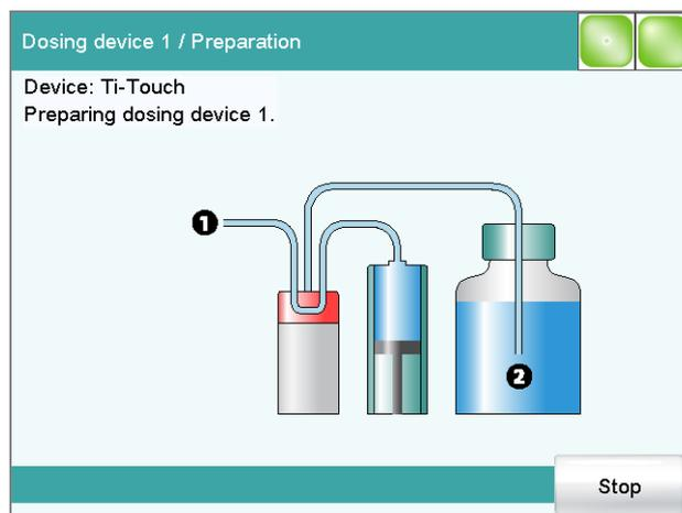
Figure 20 Live display "Preparing the exchange unit"
