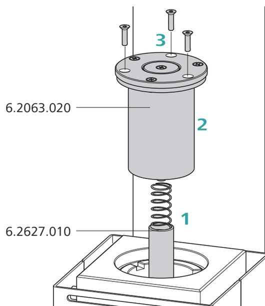
Figure 5 Mounting the sample insert
