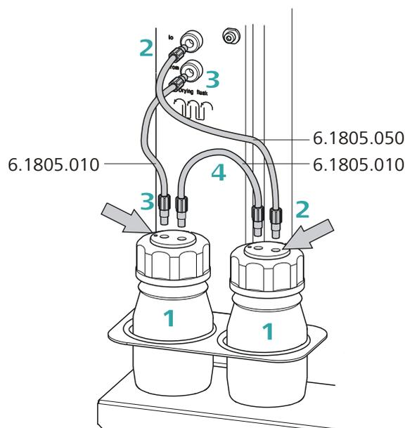
Figure 10 Mounting the tubings
