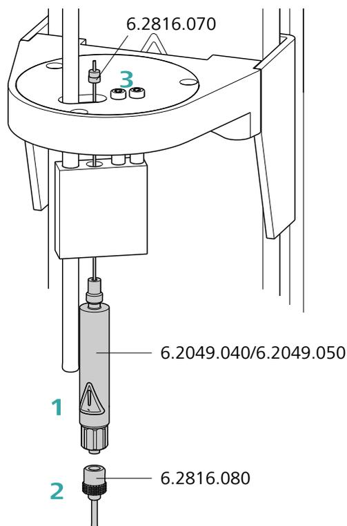
Figure 6 Mounting the needles
