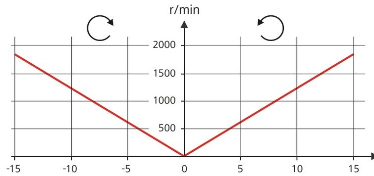
Figure 26 Rotational speed depending on stirring rate
