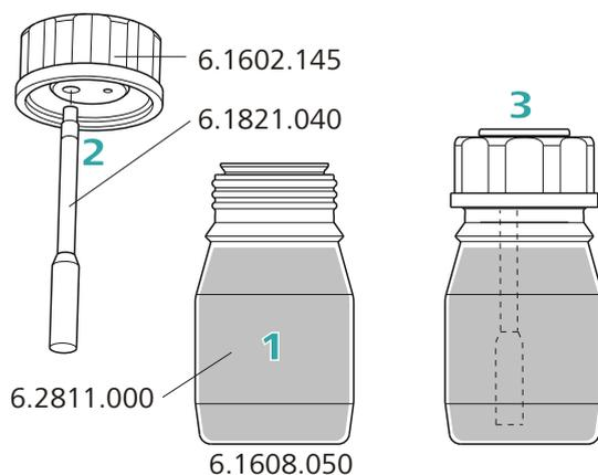
Figure 9 Preparing the drying flasks
