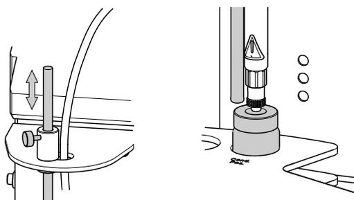
Figure 17 Adjusting the guide rod
