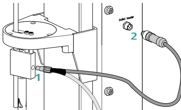
Figure 8 Mounting the heating tube
