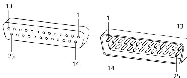
Figure 25 Pin assignment of the remote socket and plug
