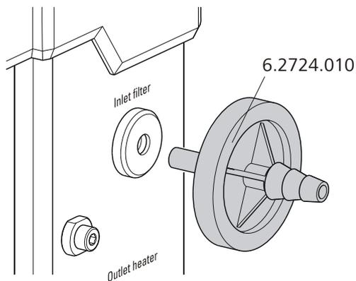
Figure 11 Mounting the dust filter
