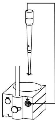
Figure 21 Rod Stirrer and titration stand
