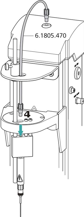
Figure 7 Mounting the tubing
