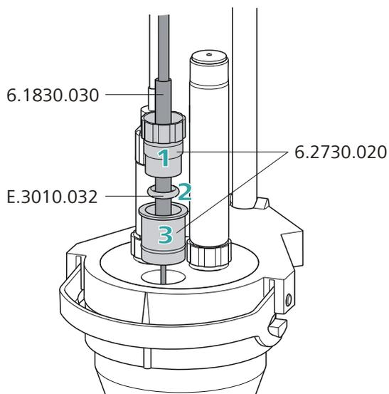
Figure 15 Volumetric KF titration cell
