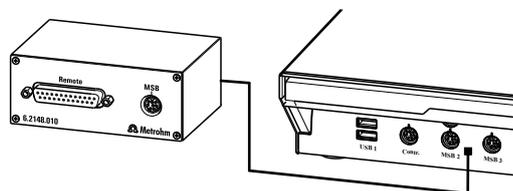
Figure 22 Connecting a remote box
