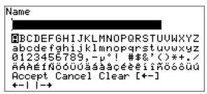
In the editing dialog for text input or numerical input, select the individual characters with the arrow keys. Use **[OK]** to apply the character in the input field. The following functions are available:
