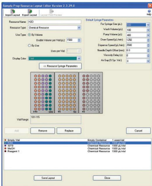
The 7696A WorkBench Software includes a color-coded **Resource Manager Screen** that lets you specify sample prep resources on trays and turrets, set default dispensing parameters, and keep track of supply levels based on volume or frequency of use.
