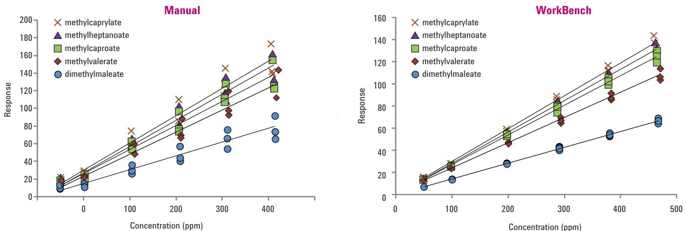
**Linear dilution: calibration curve standard preparation.** Calibration standard preparation with the 7696A WorkBench is consistently more reproducible than manual preparation.
