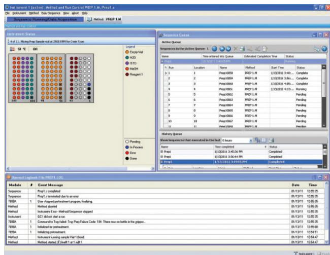
**Sample tracking:** The 7696A WorkBench generates a detailed report for each sample prepared. These reports document the date, time, instrument, and vial position, along with the steps performed and resource chemicals used – down to the vial number. An integrated bar code reader also confirms and verifies samples to ensure legal and regulatory compliance.
