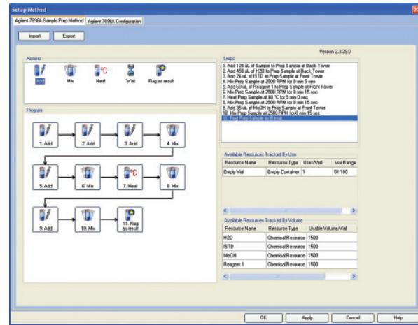
**Drag-and-drop simplicity:** With just a few mouse clicks, the WorkBench Software Method Editor Screen lets you synchronize key steps such as adding, mixing, heating, and waiting.
