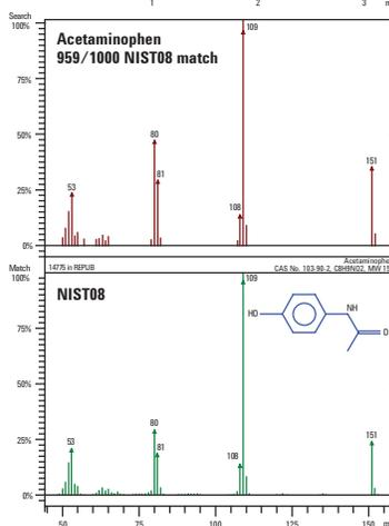
**Prompt and confident identification.** In just a couple of minutes a white powder was identified as acetaminophen using TSP and the NIST08 library. The easily accessible ionization and scanning modes of the 240 MS are great complements to TSP to quickly gain information about a sample.
