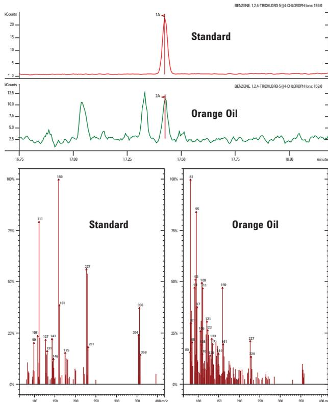
**Within the matrix, detection levels are negatively influenced by background noise. Spectral matching is also undermined by too many intense matrix ions.**
