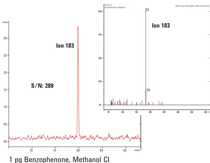
**Outstanding PCI sensitivity:** The CI full scan sensitivity is comparable to EI, so you can easily switch modes to optimize selectivity without sacrificing detection limits.
