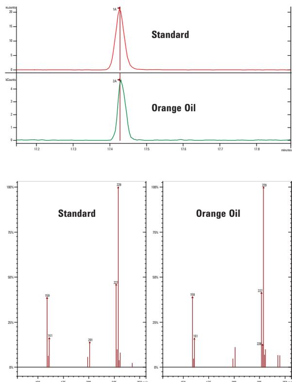
**MS/MS eliminates the matrix, resulting in a clean baseline and excellent peak shape. This significantly improves reliable quantitation of low amounts, while delivering an unequivocal spectral match for confident confirmation.**
