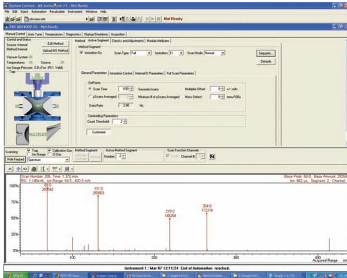
*With MS Workstation, you can easily set up, tune, and optimize all operating configurations and modes from the instrument control page.*
