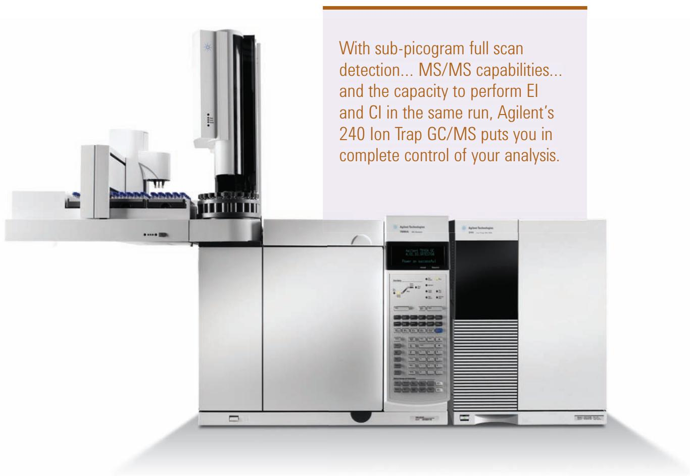
With sub-picogram full scan detection... MS/MS capabilities... and the capacity to perform EI and CI in the same run, Agilent's 240 Ion Trap GC/MS puts you in complete control of your analysis.
